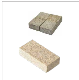
Yellow Granite 100mm wide x 100mm long & 100mm wide x 200mm long Thickness: 50mm Sawn sides, bush hammered top
