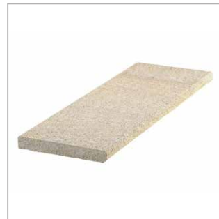
Yellow Granite 1200mm long x 400mm wide Thickness: 50mm Sawn sides, riven top, bull nosed edge
